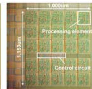
Figure 2 Nonvolatile Motion-Vector Prediction Chip: The chip is designed by using automated design tools for nonvolatile LSI. 75% of wasted power dissipation is eliminated by utilizing fine-grained nonvolatile power gating.
