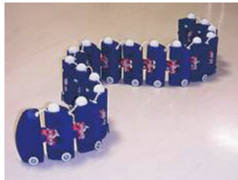
Ophiuroid robot that enables omnidirectional locomotion ( Ishiguro Gr. )
