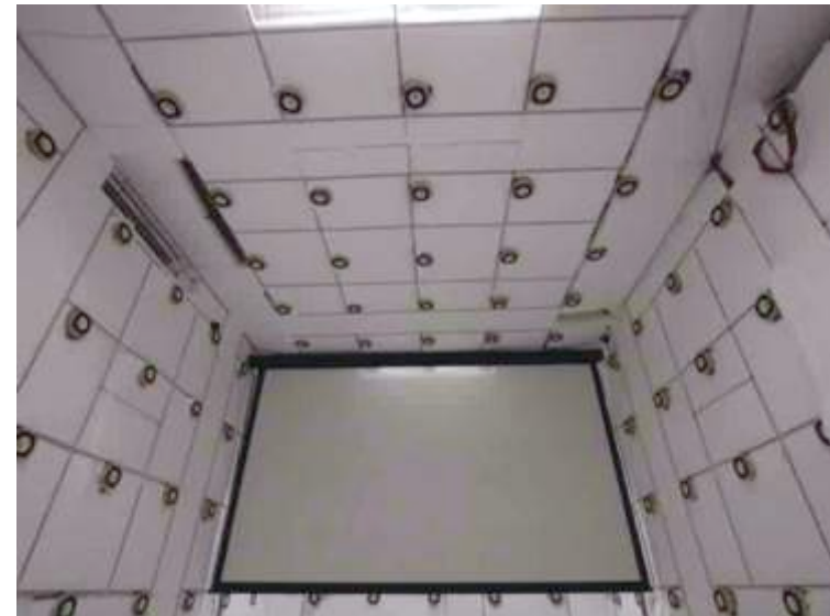
Accurate sound space communications system based on higher order Ambisonics by using 157ch loudspeaker array
