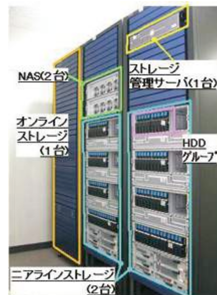
A large-scale storage system with parallel HDD operation
