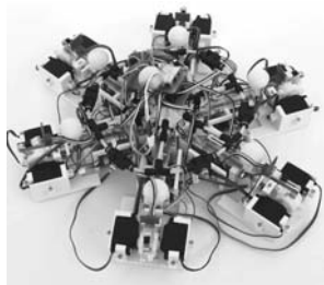
Fig.1: Soft-bodied amoeboid robot driven by a fully decentralized control scheme extracted from true slime mold
