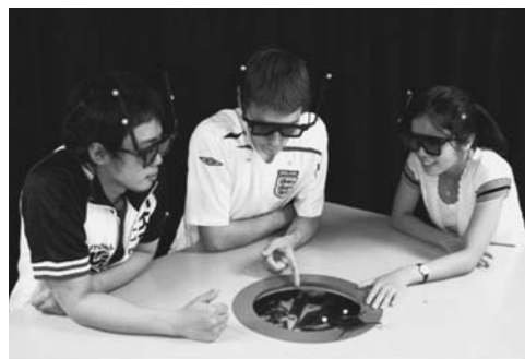
Fig. 1: Direct multi-touch interface on stereoscopic tabletop display
