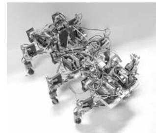
Fig.3: Hexapod robot driven by a fully decentralized neural network-based control.
