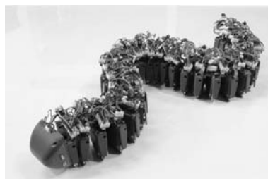
Fig.2: Snake-like robot driven by a decentralized control that exhibits adaptive scaffold-based locomotion
