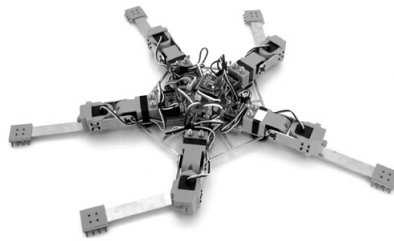
Fig.2: Brittle star-like robot that can adapt to unexpected physical damage
