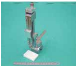
図1 グリッド式脳活動記録装置 Figure 1 Remote controllable multi-electrode manipulator
