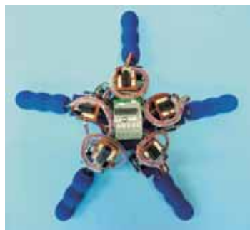
腕を自発的に役割分担して全方向移動可能なクモヒトデ型ロボット Autonomous decentralized control of a snake-like robot that exhibits highly adaptive and resilient properties.
