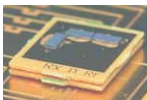
Fig.2 Ultra-small-size 3D SiP millimeter wave wireless terminal for uncompressed HDTV
