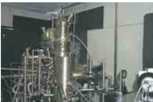
極低温 STM を備えた複合表面分析装置 Integrated Surface Analysis System with Low-temperature STM
