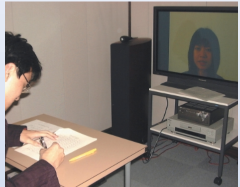
In this figure, speech intelligibility tests are performed to investigate the effect of asynchronization between talking-face movement and speech sound modified by speech-rate conversion technique.
