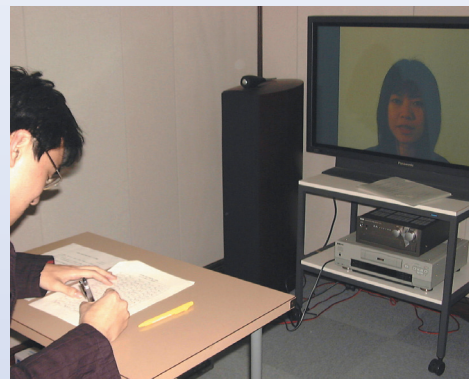
In this figure, speech intelligibility tests are performed to investigate the effect of asynchronization between talking-face movement and speech sound modified by speech-rate conversion technique.
