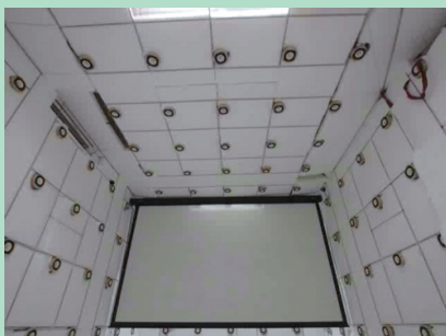
Accurate sound space communication system based on higher order Ambisonics by using 157ch speaker array
