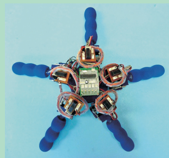
Ophiuroid robot that enables omnidirectional locomotion
