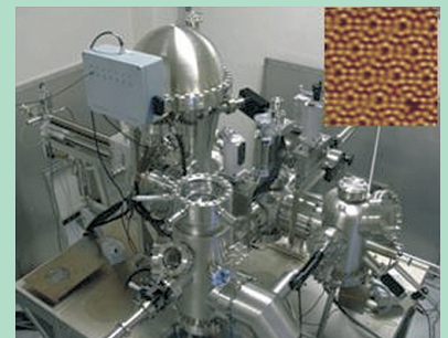
A UHV-compatible process/analyses system and the STM image of a Si surface (inset).
