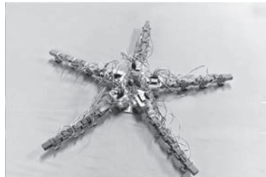
Fig.2: Brittle-star-like robot with flexible arms
