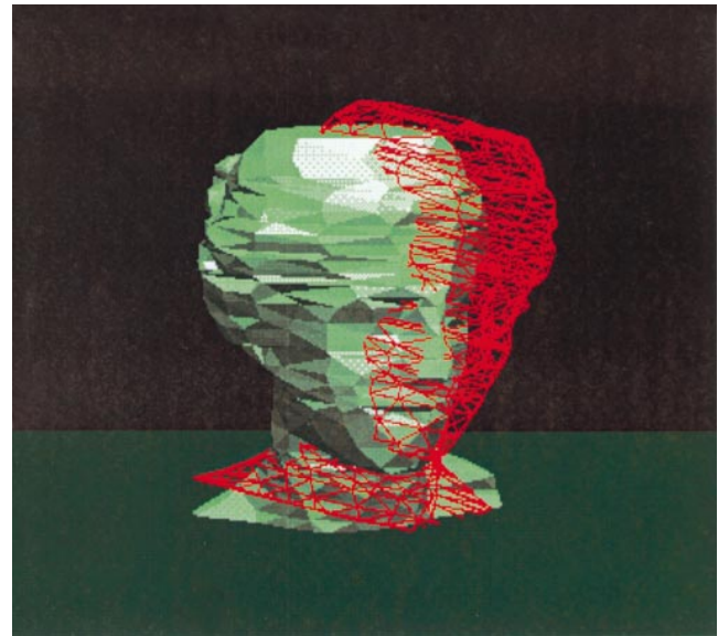
Figure 5. A snapshot of sensor and displayed object positions in the virtual object manipulation aid. Wireframe shows a sensor position, and solid object shows a displayed position.
