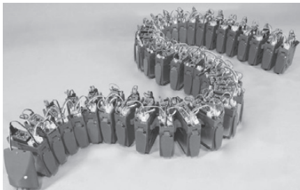
Fig.1: Snake-like robot that exhibits scaffold-based locomotion
