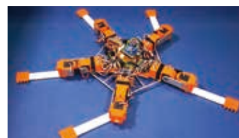
Brittle star-like robot that can adapt to physical damages
