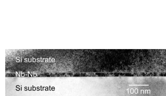
TEM cross section images of Si wafers bonded using Nb films
