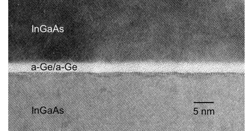
Bonding with no clear damage to the InGaAs wafer surface
