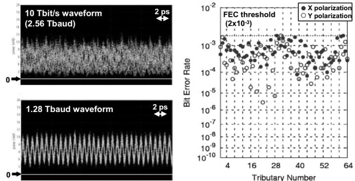
Fig. 1. 10 Tbit/s Nyquist pulse waveform and 300 km transmission result.
