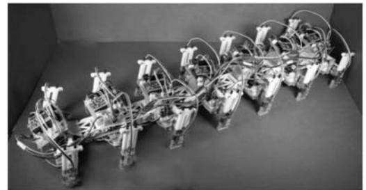
Fig.3: Sea roaches-like robot that exhibits body bending to achieve faster locomotion speed.
