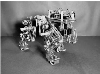
Fig.1: Quadruped robot that exhibits versatile high-speed gaits
