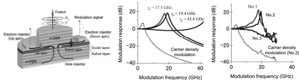
Schematic structure of spin polarization modulation VCSEL (left), calculated (center) and measured (right) responses of VCSEL under electron spin polarization modulation.
