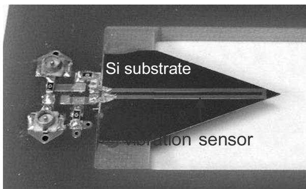
Fig. 1 Strain and vibration sensor using inverse-magnetostrictive effect.
