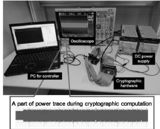
Fig. 1: Experiment for security evaluation of cryptographic hardware
