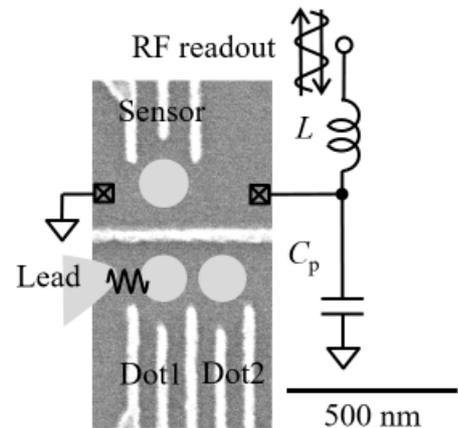
Figure: Scanning electron micrograph of the nanostructure devices
