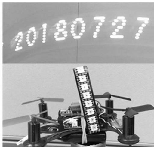
A drone race machine with LED array
