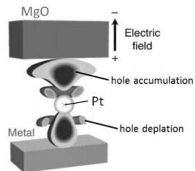
Fig. 1: Voltage-induced charge distribution of Pt atom at the MgO/Pt/Fe interface.
