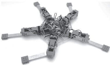
Fig.1: Ophiuroid-like robot that exhibits resilient locomotion.
