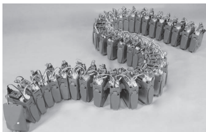
Fig.1: Snake-like robot that exhibits scaffold-based locomotion
