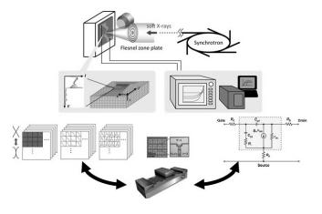
In FY2018, we succeeded in raising up high-frequenecy graphene transistor by tuning graphene/dielectric interface and quantitatively evaluating a spatial distribution of surface electron trapping of GaN-HEMT, which causes operation instabilities, so-called current collapse phenomena. Furthermore, we developed spatiotemporal operando x-ray spectroscopy, enabling spatio-temporally examining electronic states of advanced devices.
