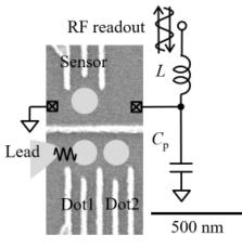
Figure: Scanning electron micrograph of the nanostructure devices
