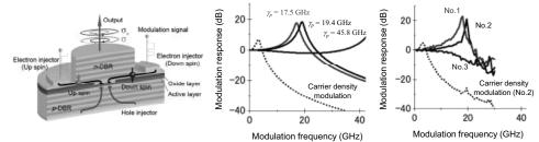
Schematic structure of spin polarization modulation VCSEL (left), calculated (center) and measured (right) responses of VCSEL under electron spin polarization modulation.
