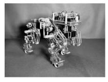
Fig.1: Quadruped robot that exhibits versatile high-speed gaits
