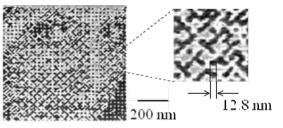
Fig.1 Digital bit data written on ferroelectric single crystal with the areal recording density of 4 Tbit/inch<sup>2</sup>.
