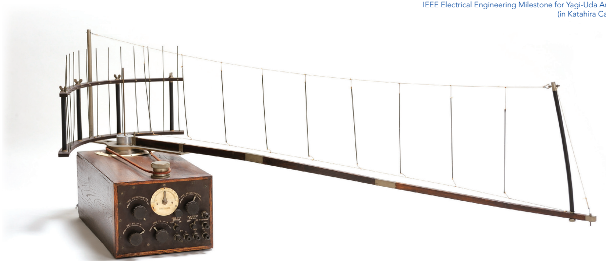
八木・宇田アンテナの実験装置 (1929) Experimental equipment for Yagi-Uda Antenna (1929)
