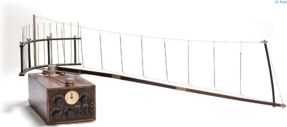
八木・宇田アンテナの実験装置 (1929) Experimental equipment for Yagi-Uda Antenna (1929)
