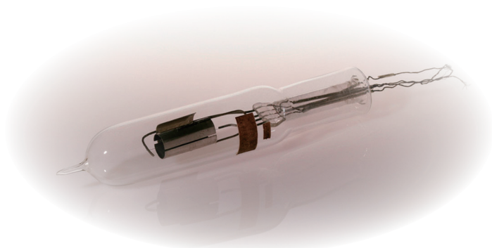
陽極分割型マグネロン (1927) Experimental equipment for Split Anode Magnetron (1927)
