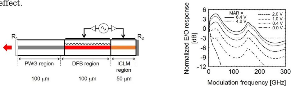
Schematic structure of a hybrid modulation laser integrated with a passive waveguide (left) and its frequency response (right).
