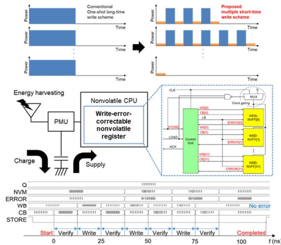
Fig. 1. Nonvolatile register based on a new data write scheme that suppresses the energy required for data retention in intermittent computing.
