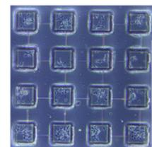
Neuronal circuits formed in a microfluidic device
