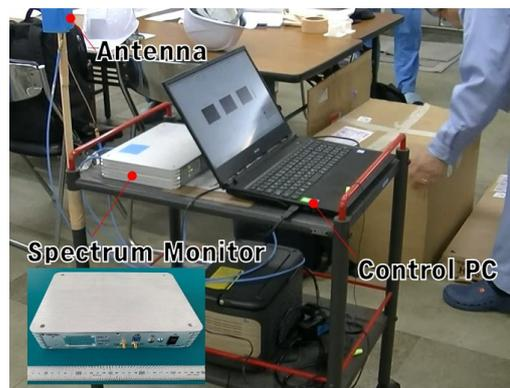
Fig.2: Factories Radio Environment Monitoring
