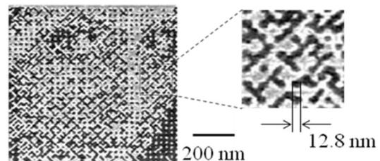
Fig.1 Digital bit data written on ferroelectric single crystal with the areal recording density of 4 Tbit/inch<sup>2</sup>.
