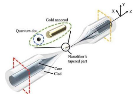
Fig. 1. Plasmon-enhanced single photon source on an optical nanofiber.
