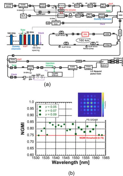
Fig. 1. 1 Tbit/s/λ PS-32 QAM coherent Nyquist pulse transmission over 1,600 km. (a) Experimental setup, (b) transmission results.
