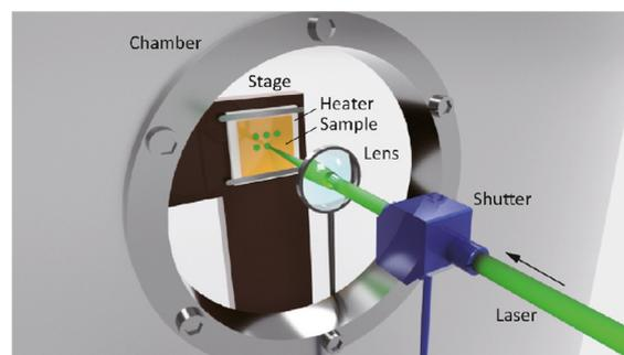
Fig. 2. Magneto-optical materials used in magnetic sensors and optical communications were fabricated using localized laser heating. This enabled the integration of magneto-optical materials with semiconductor circuits and optical circuits.
