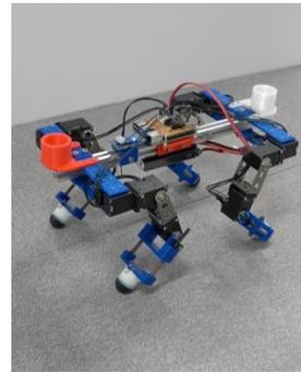
Fig.2: Quadruped robot that realizes a turning gait according to the center of mass position
