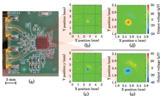
Fig. 1. Measurement of the leakage magnetic field distribution generated by a commercial analog high-frequency circuit. This method revealed a significant leakage magnetic field in the central part of the chip.
