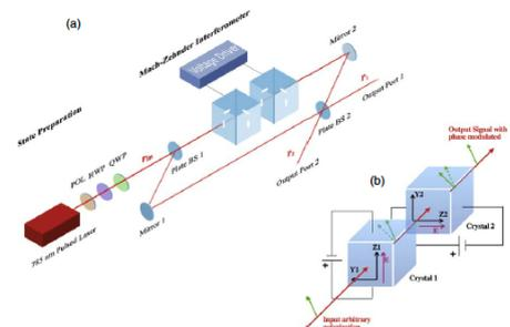
Fig. 2. Ultra-low-loss polarization-maintaining optical switch.
