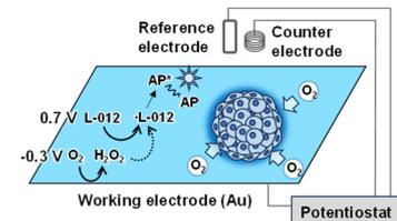
Electrochemiluminescence imaging of a cellular spheroid
