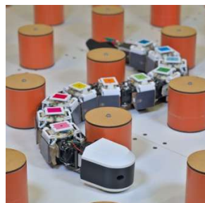
Fig.2: Amphibious locomotion of an eel-like robot via decentralized control
